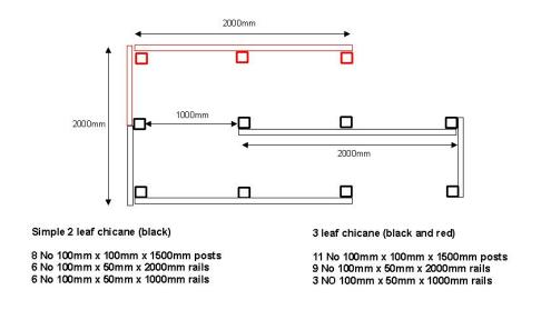
Example of an 'Accessible' Chicane. The only difference to make it accessible is that the enclosed space at the end would have to be 2m long instead of the 1m shown in the drawing. This does mean that it would be accessible by motorcycles.
